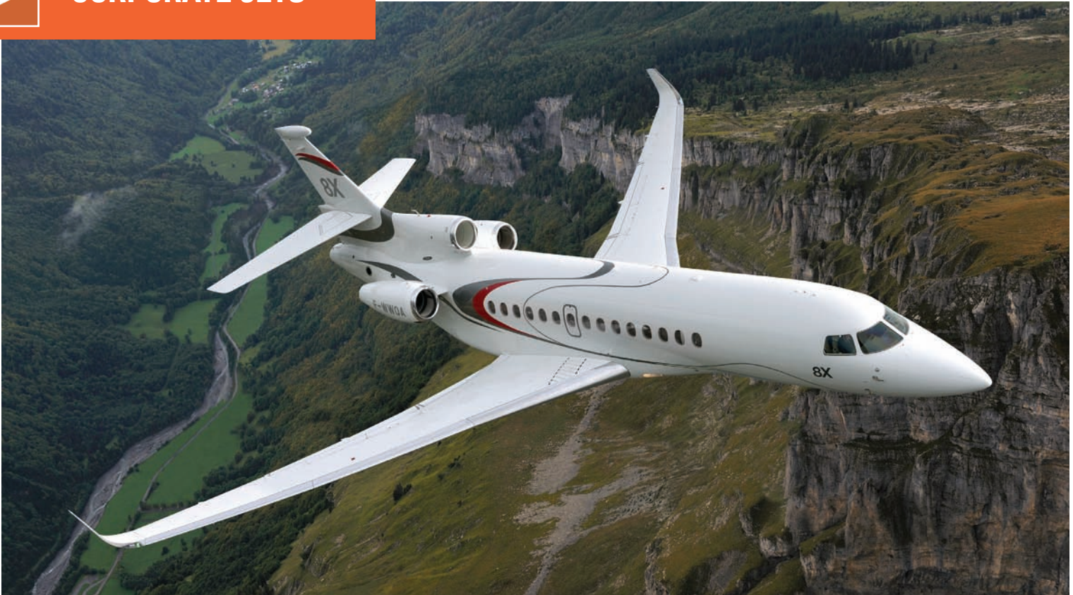
The Dassault 8X has a range of 6,540 nautical miles of range and can easily connect Cape Town with different points in Europe.
