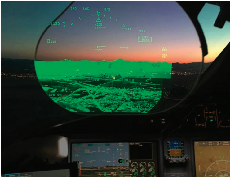
The 8X features the business jet world's first Combined Vision System – the FalconEye
