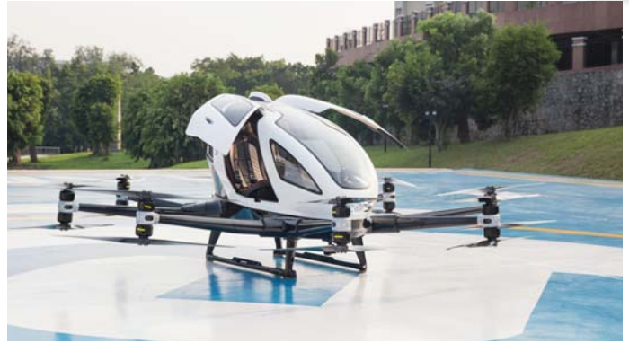
The EHang 216-S, a two passenger eVTOL multicopter production model aircraft made for advanced air mobility (AAM), was awarded the 'type certification' last year by the Civil Aviation Administration of China last year – making it the first in the world.
