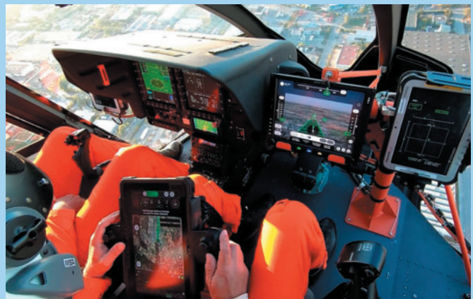
The Airbus Helicopters' FlightLab flew fully automated from lift-off, taxi, take off, cruise, approach and then landing during a one-hour test flight by following a predefined route. Photo credit Airbus.
