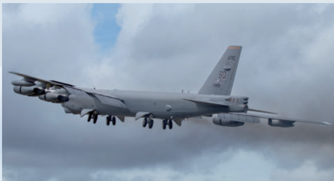
The venerable Boeing B-52H Stratofortress climbs away into the sky with its eight engines leaving a trail of smoke in the sky.
