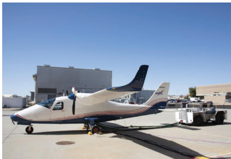
As far back as 2021 NASA's all-electric X-57 Maxwell aircraft underwent high-voltage ground testing at NASA's Armstrong Flight Research Centre in California. The aim of the X-57 project is to help the Federal Aviation Administration set certification standards for emerging electric aircraft markets. Photographer: NASA/Lauren Hughes.
