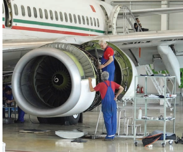
Boeing 737 MRO. Earlier in 2012 Aerostar's biggest MRO client from Africa was Royal Air Maroc. Here a RAM Boeing 737 underwent a 'C' check.
